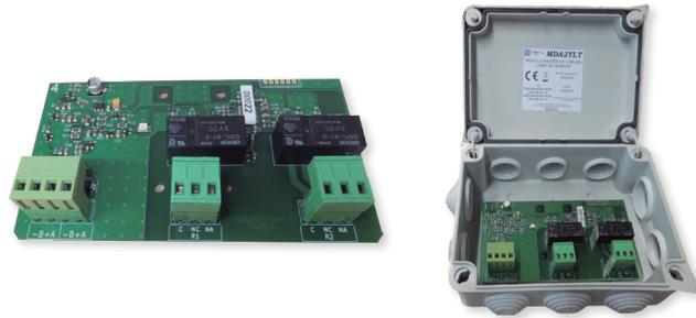
Microprocessed and algorithmic-addressable module (with short-circuit insulator) which is installed as one more element in the loop.
